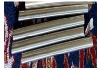
Figure 3. Iron based SMA (Fe Mn Si Cr Ni)
