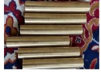
Figure 2. Copper based SMA (Cu Ni-Al Fe)
