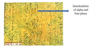
Figure 10. Microstructure image of SMAs
